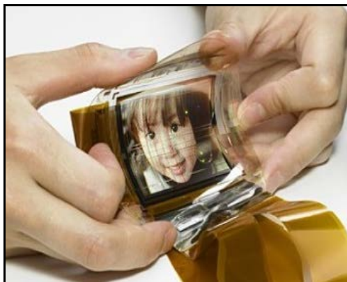
Figure 7: OLED ultra-flat deformable screen (by Sony).
