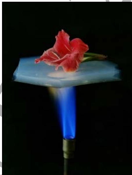
Figure 6: Aerogel, the part on which there is the flower is at room temperature, despite the direct contact of the flame.
