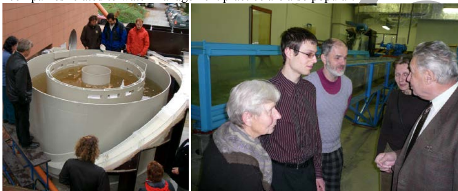
Fig. 1: Physical model of a double rain separator on a length scale of 1:10 and a trainees lifelong learning course.
